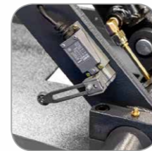
CE-Stop (foot protection) 下限位开关 (防压脚设 计)
